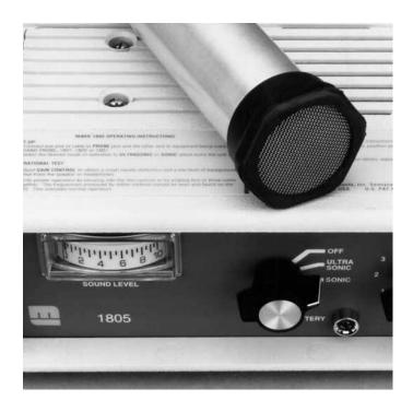
The Dielectric 1805 Multisonic Detector pinpoints leaks in pressurized cable systems by converting both sonic and ultrasonic sounds into visual and audible signals. Designed to span the range of frequencies from 100Hz to 100kHz, the Model 1805 quickly detects both large and small pressure leaks. Unique circuitry enhances leak sounds while diminishing unwanted background noises. A sensitive meter responds to low signal levels cueing the user to listen for difficult to detect leaks.
