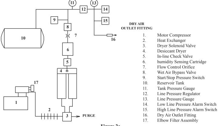
Figure 2c Flow Schematic for Model 200"C" Dryers
