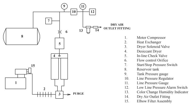
Figure 2a Flow Schematic for Model 200"A" Dryers
