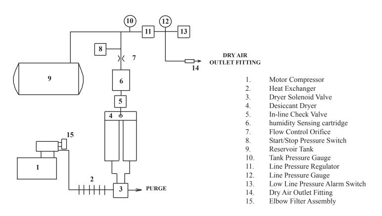
Figure 2b Flow Schematic for Model 200"B" Dryers
