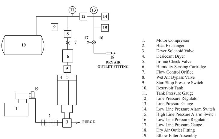
Figure 2d Flow Schematic for Model 200"D" Dryers
