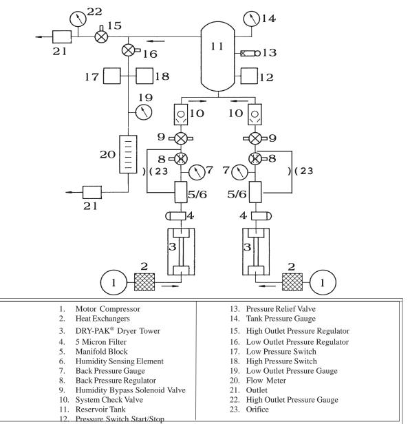
Figure 2 Air Flow Diagram
